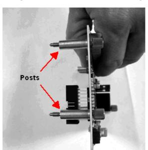
2. Pick up the Add-On Board and notice the four posts on the bottom.
